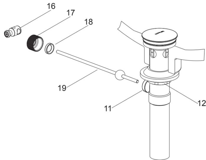
Remove the latch(16) and retaining nut(17). Fit the plastic washer(18) and retaining nut onto the ball lever(19). Insert the ball lever assembly into the drain lever hole and through the stopper hole. Tighten the retaining nut.
