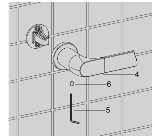
Slide the main body(4) onto the bracket. Orient the screw hole downward. Tighten the screw(6) with the hex wrench(5).
