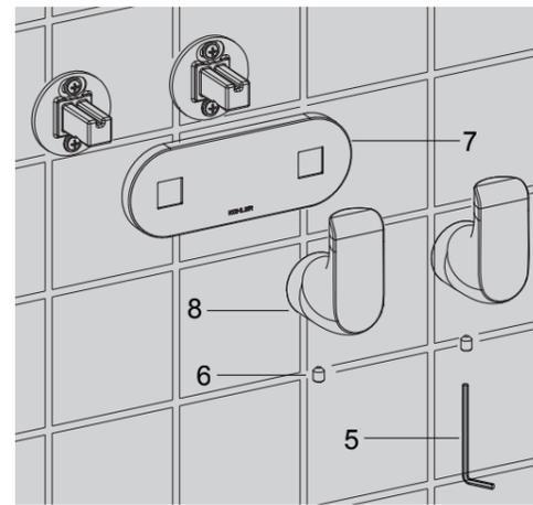
Slide the escutcheon(7) onto the bracket. Keep "KOHLER" logo on escutcheon is on positive direction. Slide the robe hook(8) onto the bracket. Orient the screw hole of the robe hook downward. Tighten the screw(6) with the hex wrench(5).
