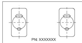
Select a location on the vertical wall to stick the templet, ensure the templet is horizontal. Drill hole in the finished wall as required.
