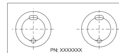
Select a location on the vertical wall to stick the templet, ensure the templet is horizontal. Drill hole in the finished wall as required.
