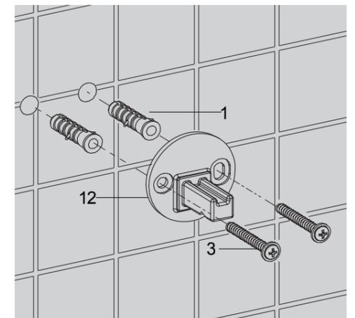
Press the anchor(1) into the hole. Orienting the groove of the bracket upward. Secure the bracket(2)(12) with the self-tapping screw(3).
