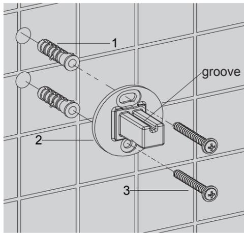
Press the anchor(1) into the hole. Orienting the groove of the bracket upward. Secure the bracket(2) with the self-tapping screw(3).
