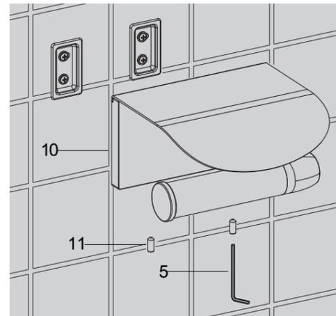
Slide the main body(10) onto the bracket. Orient the screw hole downward. Tighten the screw(11) with the hex wrench(5).
