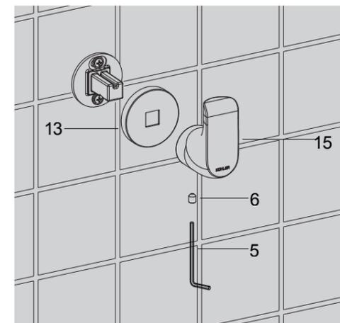
Slide the escutcheon(13)(14) onto the bracket. Orient the gap of escutcheon(14) downward. Slide the main body(15)(16) onto the bracket and keep the screw hole downward. Tighten the screw(6) with the hex wrench(5).
