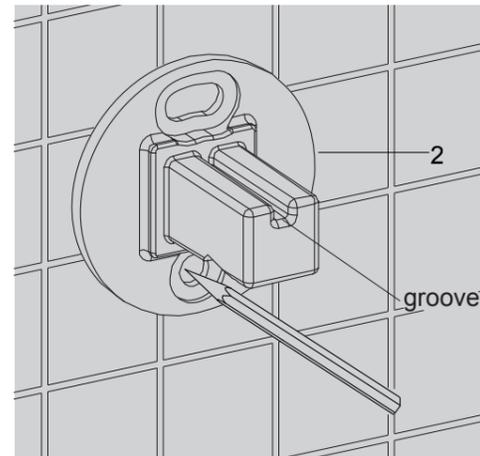
Select a location on the vertical wall to install the bracket. Mark anchor(1) mounting hole location on wall, ensure the groove of bracket(2)(12) upward. Drill hole in the finished wall as required.
