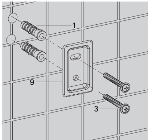
Press the anchor(1) into the hole. Orienting the large slotted mounting hole of the bracket upward, the smaller hole of the bracket downward and two screw holes are vertical. Secure the bracket(9) with the self-tapping screw(3).
