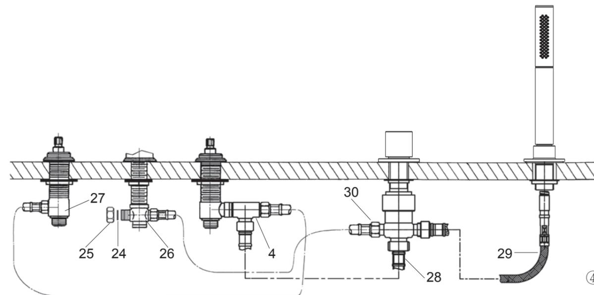
Put the fiber washer(24) into the plug(25), Tighten the plug to one of the ports of the center tee(26) for the spout.
