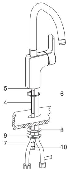
From underside of the sink, place the washer(8), washer(9) and the nut(10) . Position the faucet so that the handle is on the right side. Tighten the nut to secure the faucet to the sink.
