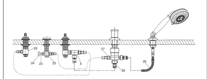
Put the fiber washer(23) into the plug(24), Tighten the plug to one of the ports of the center tee(25) for the spout.
