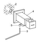
To perform installation, installer must provide G1/2" female supply fitting(1).
