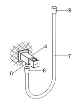
Apply a ring of plumbers putty or other sealants to the kit(4) base. Install the kit onto the outlet bush(2), adjust the kit to the outlet(6) downwards. Tighten the screw(5) in the bottom of the kit by the hex wrench. Remove any excess putty.
