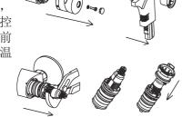
Very hard water can obstruct the filters protecting the thermostatic cartridge and reduce the flow of water. Clean the filters by soaking the thermostatic cartridge on which they are restrained in hot vinegar and follow the instructions in the figures on removing the cartridge(The 37 mark is aligned with the mark on the body before removing.)
