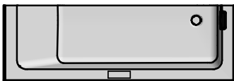
Keypad Location Size: 5.75" X 1.75" Centred on Side Deck (Keypad available when paired with Enhanced Bathing Options)
