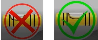
6. The leveled and supported tub (adjustable feet or grout/mortar), should also have the **apron in contact with the floor throughout its length**. In case the floor is not leveled and part of the apron is not touching the floor, it's a must to shim the apron and fill the gap with a structural material like wood or plastic. The distance between shims should not exceed 6" and the max. gap to shim should not exceed 1/4".
