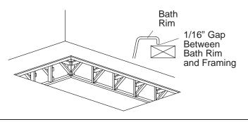
5. Sunken Installation (oval models): Carefully position the bath face down in the desired installation location. Draw a line around the entire edge. Measure in from the line 3/4", and draw a second line. This is your cut line. Cut out by following the cut line. Make sure the bath will be supported by the bath base, not the rim. Do not hang the bath by the rim.
