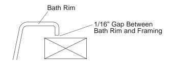
Option For Sunken Installation: Set the bath into the sunken installation. Make sure the unit is level and is resting on the bath base. Insert the drain tailpiece into the trap. Apply a bead of silicone sealant under the rim of the unit.
