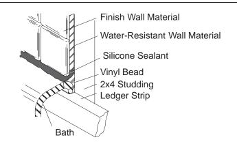
For installations that do not use a vinyl bead, cover the framing with water-resistant wall material as shown. Seal the joints between the bath rim edge and the wall material with silicone sealant.
