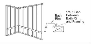
Recess Installation: The suggested stud construction is illustrated.
