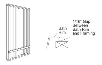
4. Sunken Installation (excluding oval models): The suggested stud construction is illustrated. Refer to the roughing-in document packed with the bath. Do not hang the bath by the rim.
