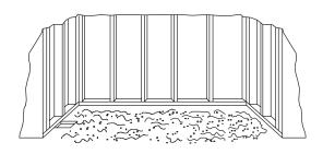
**Option For Using Construction Adhesive: Apply** a generous amount of construction adhesive to the bottom of the base. Set the bath in the desired location, and level it.
