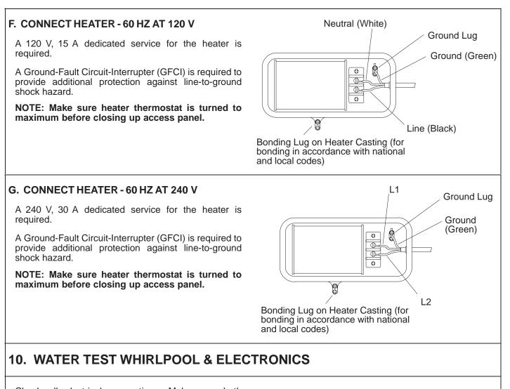
Check all electrical connections. Make sure both connections to the pump are securely tightened.
