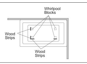
3. **Sunken Installation:** Set unit into sunken installation. Make sure the bath/whirlpool is level and is resting on all blocks. Insert the tailpiece into the trap. Apply a bead of RTV sealant under rim of the bath unit.
