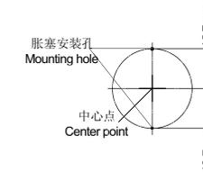
Mark anchor(5) hole locations vertically 12.7mm above and below the center points as shown. Drill holes in the finished wall as required.
