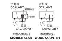
Note: waterproof unprotected overhang area on the underside of wood counter.
