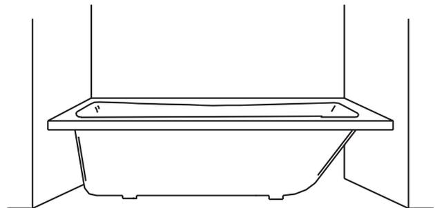
Use 25~30 Kg dry cement and sand mix. Add water to make a paste mortar. Remove the tub. Cover the installation area with the mortar starting from the middle of the tub as shown. The height of the mortar should reach the bottom of the tub.
