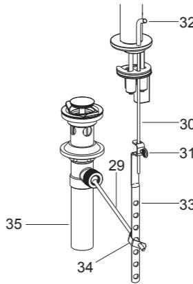
**NOTE:** Do not reposition the drain after the locknut is tightened, or you may break the putty seal.
