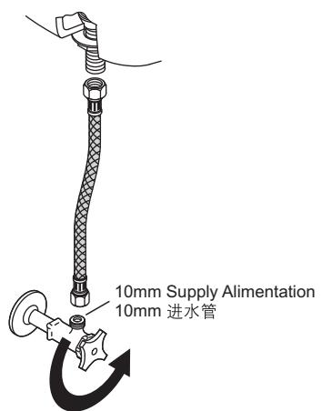
**11** Flush several times and check for leaks.
