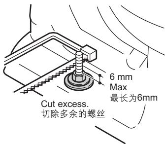
**6 Install floor mounting kit as shown in the figure. Do not overtighten.**
