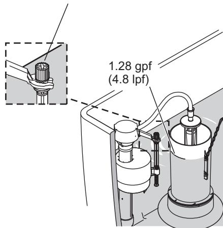
**13** Install the tank lid and the seat. Use the supplied 1/4"-20 seat bolts and washers. Periodically check for leaks for several days following the installation.
