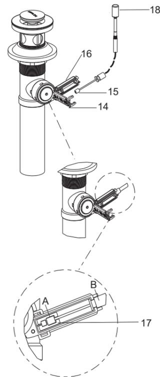
Open the coverplate(14) on the drain body, and insert cable end(15) into the square hole (17) of cable box(16). Make sure the cable is properly buckled at both ends(A, B) of the cable box as the figure shown.
