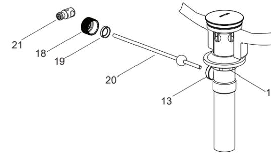
Remove the latch(21) and retaining nut(18). Fit the plastic washer(19) and retaining nut onto the ball lever(20). Insert the ball lever assembly into the drain lever hole and through the stopper hole. Tighten the retaining nut.
