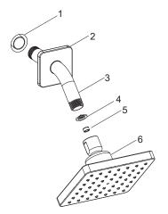
Apply a ring of plumbers putty at the backside of the escutcheon(2). Slide the escutcheon onto the shower arm(3). Apply tape or thread sealant to the shower arm threads, and install the shower arm into the supply fitting or connector(1, not provided).
