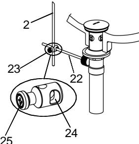
Insert the ball lever rod(22) into the bigger hole(24) of the latch(23). Insert the lift rod into the other hole of latch. Position the lift rod, ensure the distance between lift rod knob and the body is about 10mm. Push the ball lever rod down to the open position. Tighten the screw(25) on the latch.
