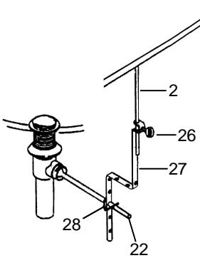
According to the lift rod length, bend the link(27). Connect the link onto ball lever rod with 'V' clip(28). Slide lift rod(2) into the hole on link. Position the lift rod, ensure the distance between lift rod knob and the body is about 10mm. Push the ball lever rod down to the open position. Tighten thumb screw(26).
