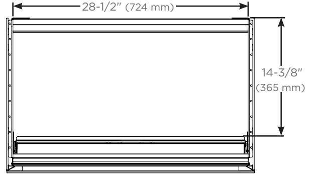
Top view for plumbing and sink clearance
