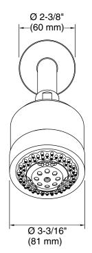
Technical InformationAll product dimensions are nominal.Drain included:NoDrain withNooverflow:Showerhead/Body Spray:Rated maximum1.75 gal/min (6.6 l/min)flow:Pressure:80 psi (5.5 bar)
