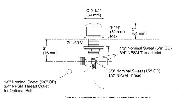
Can be installed in a wall-mount application to the same roughing-in dimensions.
