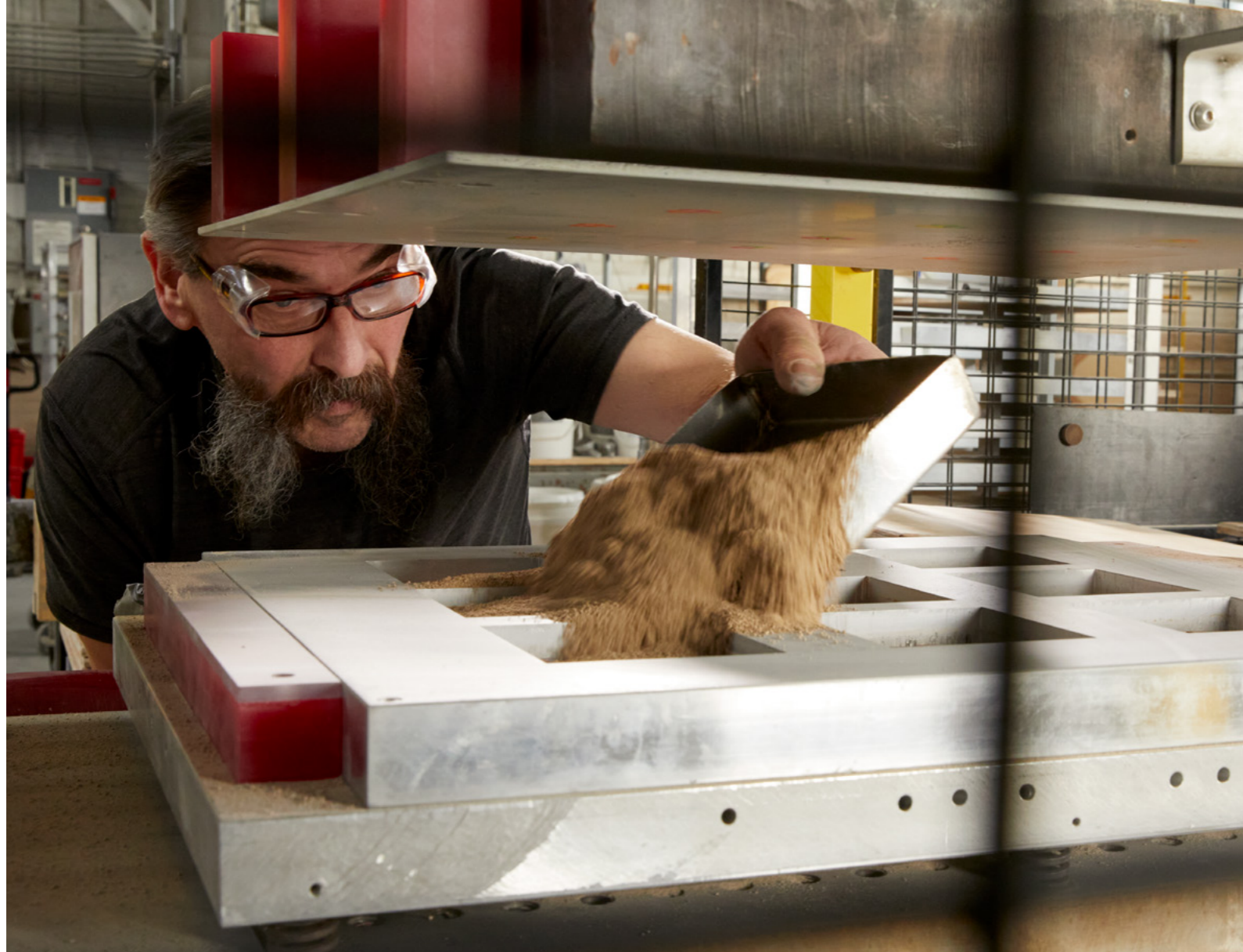
A KOHLER WasteLAB™ team member preparing to press a new batch of tile.
