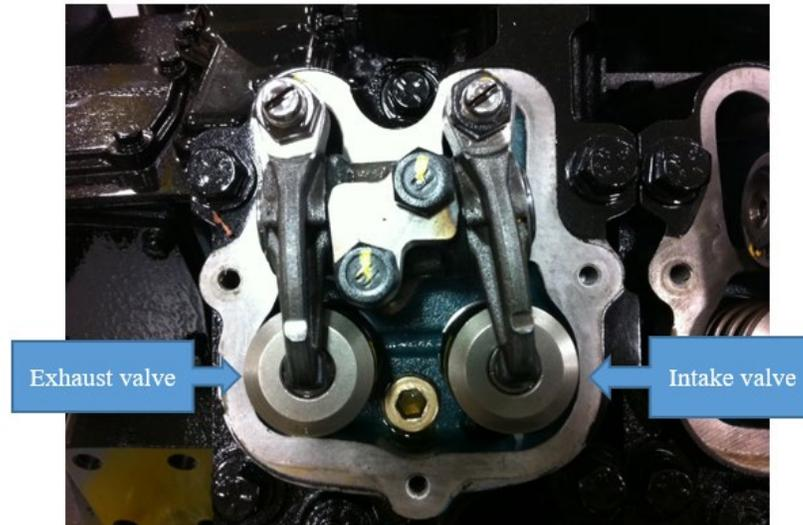
5. Once the proper angle is set, use the screwdriver to hold the adjuster in place while tightening the locking nut to 36 lb/ft with a 17mm wrench. Torque the nut to 36 lb/ft.
