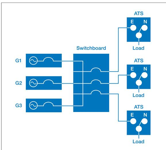
**CONFIGURATION 3 – SWITCHBOARD WITH A BREAKER PAIR PER GENERATOR**
