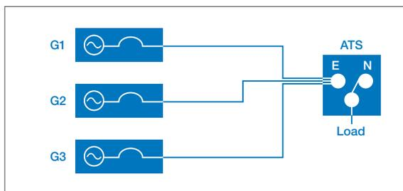
A power distribution block setup could be used; if this is built into the ATS, it must be included within the ATS UL1008 listing. If installed externally to the ATS, it must meet NEC installation guidelines.
