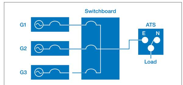
If the switchboard is within line of sight of the generators, a bus bar could be located on the generator with a single EOB per generator in the switchboard. Overall, this is the most flexible design, and allows for expansion with good future planning.
