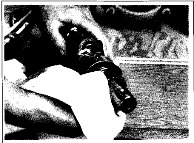
Figure 10-2. Heat Sprocket Before Installing.
