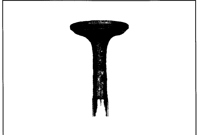
Stem Corrosion: Moisture in the fuel, or condensation are the most common causes of valve stem corrosion. Condensation occurs from improper preservation during storage and when engine is repeatedly stopped before it has a chance to reach normal operating temperatures. Replace corroded valves.
