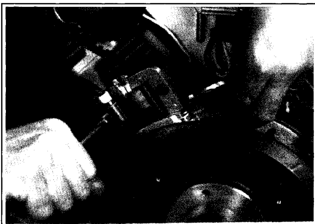
Figure 11-38. Adjusting Air Gap of Ignition Modules.
