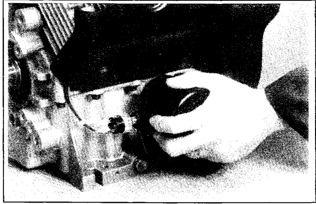
Figure 6-6. Hand Tighten New Filter in Clockwise Direction.
