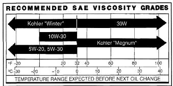
Figure 2. Viscosity Grades Table.
