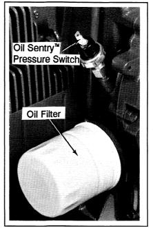
Figure 6. Oil Filter and Optional Oil Sentry™ Switch.
