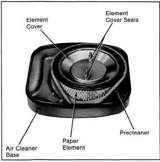
Figure 7. Air Cleaner Housing Components.
