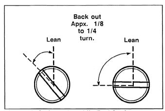
Figure 12. Optimum Low Idle Fuel Setting.
