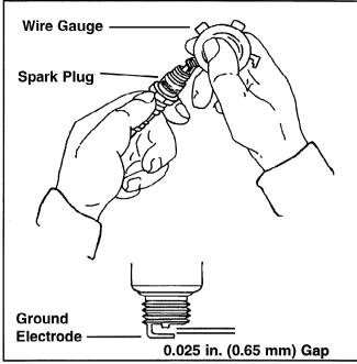
Figure 8. Servicing Spark Plug.
