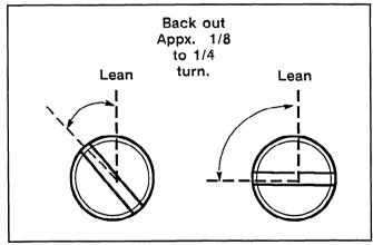
Figure 11. Optimum Main Fuel Setting.
