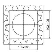
The size of openning on the tile is as the figure shown. Lay the tile.
