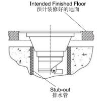
Determine the height of prearranged stub-out according to the diameter of stub-out and the height of intended finished floor.
