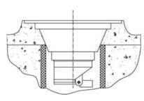
Mount the floor drain according to the Determined height. Position it. Fill up the interspace around it with cement.
