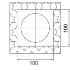
Mount the floor drain according to the determined height. Position it. Fill up the interspace aroud it with cement.
