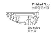
To drain easily, the mounting position of floor drain must be at the lowest area of the whole finished floor.
