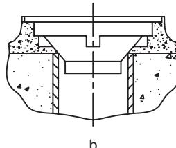
4. Level the drain and install it according to the pre-decided installation height. Caulk the surrounding gaps. Refer to Fig.b.
