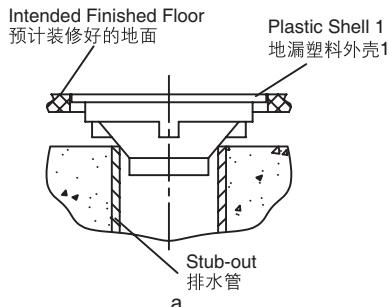
3. Take out the drain body, cover and core. Put the plastic shell into the pipeline and then caulk the gap with pre-blended cement and mortar (1:1). Refer to Fig.b.
