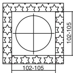
6. Caulk the gap with cement and then clean the excessive cement.
