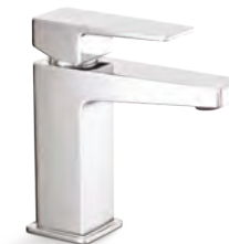
Honesty Cold Water Single-Hole Single-Control Lavatory Faucet K-24747X-4CD-CP • Reach: 105 mm Height: 151 mm • Directionally adjustable aerator • Water saving 40% according to LEED standard • Includes supply hose
