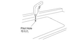
Cut along the outline to cut out the opening in the countertop. 沿着画出的轮廓线切出水槽安装孔。
