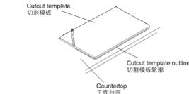
Trace the outline of the cutout template on the countertop with a pencil at the desired installation location. 用铅笔在厨房工作台上您希望安装水槽的位置画下切割模板的轮廓。
