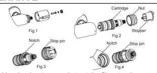
Very hard water can obstruct the filters on the thermostatic cartridge and reduce the flow of water. Please clean the cartridge as follows: Shut off the water supply of the faucet and open the water flow handle, then proceed to remove the cartridge. The cartridge is sense organ, please be careful.
