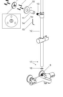
Tighten the screw(17) with hex wrench.
