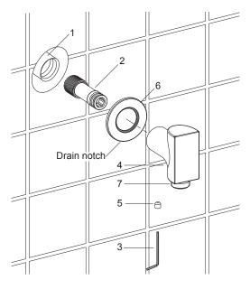
Before installation, plumber must provide G1/2" female supply fitting(1).
