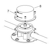
Secure protector(8) onto the base with screws(7).
