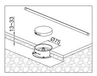
Make sure the distance between bottom of protector and top surface of tiles is within 13~33mm(top surface of tiles is between the MIN and MAX line on the protector). Drill Ø75 hole on the tile. Lay the floor tiles. Cut away the extending part of protector in accordance with the tile surface before install the faucet. The faucet's installation refer to the corresponding installation instructions.
