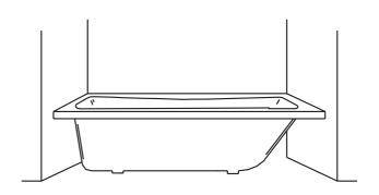
Use 25~30 Kg dry cement and sand mix. Add water to make a paste mortar. Remove the tub. Cover the installation area with the mortar starting from the middle of the tub as shown. The height of the mortar should reach the bottom of the tub.
