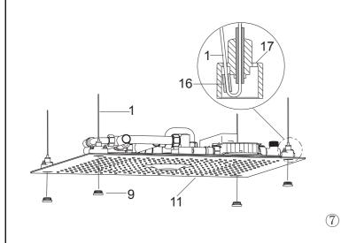
After connecting the hoses, push the shower head(11) upward by dragging the stainless steel wires, until the shower head presses against the suspended ceiling and all stainless steel wires are stretched tight. Make each wire sleeved with a clip(16) go through the hole(17) to hide the exposed length of it. Press the cap (9) along with an O-ring into each corner hole on the shower head.
