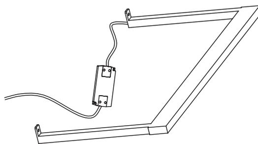
6. If installed together with Kohler Be Box cabinet, the light shall be installed inside cabinet top. The wire can be fixed with double-sided adhesive tape.
