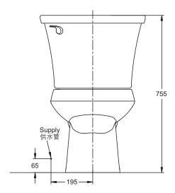
Important: Toilet must have 305mm/400mm minimum roughing-in to install properly.
