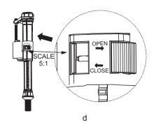
Float adjustment instructions: Make sure the height of surface E is 2-4mm lower than surface G. 浮桶调节注意事项: 调节螺杆时保证E面下沉于G面2-4mm。
