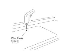
Cut along the outline to cut out the opening in the countertop 沿着画出的轮廓线切出 水槽安装孔。
