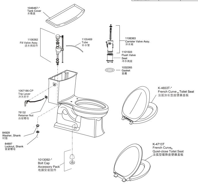
订购时请说明颜色代码(-\*)或表面处理(-\*\*) Color code (-\*) or finish (-\*\*) must be specified when ordering. 盖板的维修零件请详见盖板的维修零件图。 Please refer to service parts page packed with seat for detailed seat service parts.
