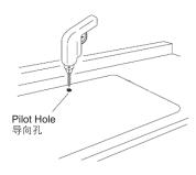
Cut along the outline to cut out the opening in the countertop 沿着画出的轮廓线切出 水槽安装孔。
