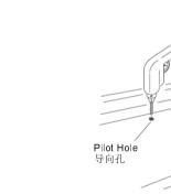
Trace the outline of the cutout template on the countertop with a pencil at the desired installation location 用铅笔在厨房工作台面上您希望 安装水槽的位置画下切割模板的轮廓。
