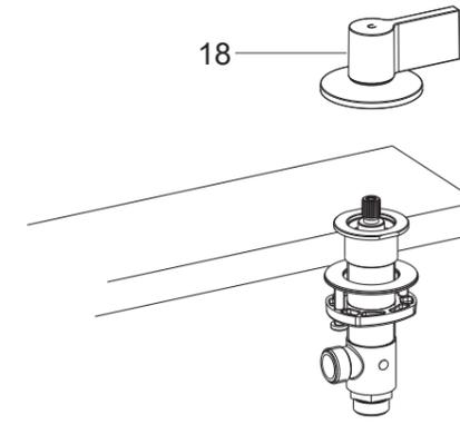
Ensure the valves and handles are in the off position.
