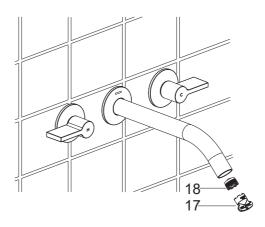
Ensure that all coupling nuts are tight. Ensure that the handles are in the off position.
