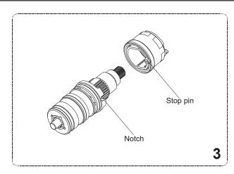
3. After cleaning, install the "stop assembly" back on the cartridge, adjust the stop pin into the notch.
