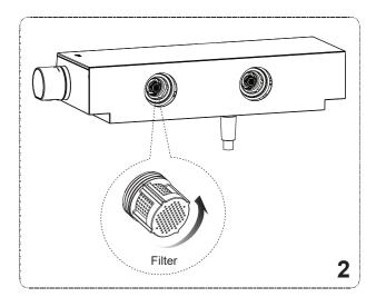
2. Rotate counter-clockwise 90° to take out the filters. Clean the filters by soaking them in warm vinegar. Reinstall them in turn.
