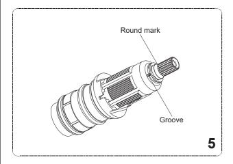
5. **NOTE:** Do not turn the cartridge when reinstalling it. If you turned it accidentally, you should adjust it and be sure that the round mark is correctly in line with the groove, or readjust as per the steps of verification and setting.
