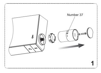
1. Before your action, make sure the number 37 on the temperature handle is upward vertically(It could not be turned counter-clockwise if not pushing the button). Remove the handle kit.
