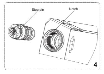
4. Install the assembly cartridge and stop in the body, adjust the stop pin into the notch.
