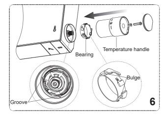
6. Install the bearing(without turning the spindle). Make sure the bulge of the bearing align with the groove of the body. Install the temperature handle. Make sure the number 37 on the temperature handle is upward vertically(After assembly, it could not be turned counter-clockwise if not pushing the button). Tighten the screw with washer. Install the handle plug.
