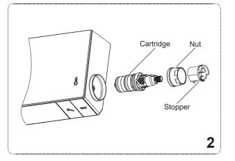
2. Unscrew the nut and stopper. Remove the cartridge cautiously. Clean the thermostatic cartridge by soaking it in warm vinegar.
