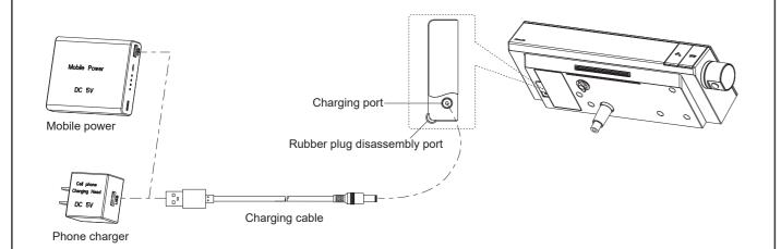
Connect the charging port(visible by opening the rubber plug) with 5V DC power supply(such as mobile power or phone charger) via charging cable.
