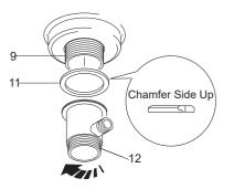
Install the seal(11), secure and tighten the drain body(12) to the waste by hand.
