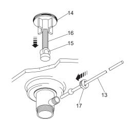
Adjust the drain body to enable the ball lever(13) and lift rod(8) to engage.
