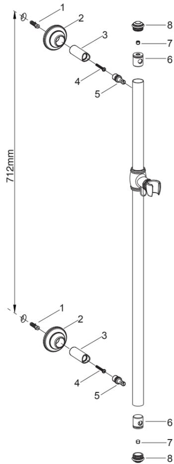
Select a suitable location to drill two holes on the finished wall according to the rough-in dimensions and diameter of the anchor(1), their distance is 712mm. Press the anchors into the holes.
